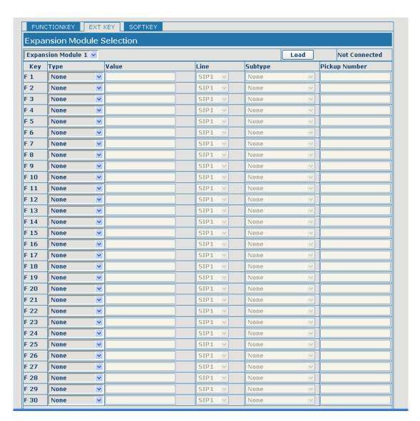
**EXT KEY** has the same usage with the Function key. "In" port connects the phone, "Out" port connects the next one, if there is only, you don't need for power supply, if there are more than one, you need supply 5V power for the first one, and use RJ-45 direct connector.
