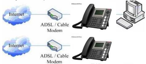
Shared network connection—Use this method if you have a single Ethernet port in your workspace with your desktop computer already connected to it. First, disconnect the Ethernet cable from the computer and attach it to the WAN port on the back of your phone. Next, use the Ethernet cable in the package to connect LAN port on the back of your phone to your desktop computer. Your IP Phone now shares a network connection with your computer. The following figure is for your reference.
