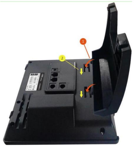
C. It is the right picture after fixing the stand bracket below:
