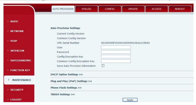
The equipment supports PnP, DHCP, and Phone Flash to obtain configuration parameters. They will be queried in the following order when the equipment boots.
