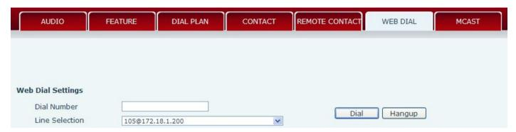
This feature allows a call to be initiated by a computer. To place a call, enter the number in the Dial Number box, select the line in the Line Selection box and press the Dial button. To end the call, press the Hang-up button.
