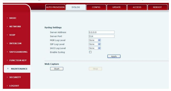
Syslog is a protocol used to record log messages using a client/server mechanism. The Syslog server receives the messages from clients, and classifies them based on priority and type. Then these messages will be written into a log by rules which the administrator has configured.
