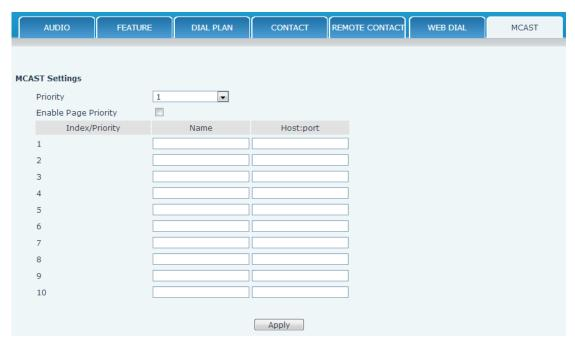
Use the multicast function to send notice to every member of the multicast is simple and easy. By setting the multicast key on your phone, you can send multicast RTP flow to the pre-configured multicast address. By listening multicast address is configured on the phone, listen and play the multicast address to send the RTP stream.
